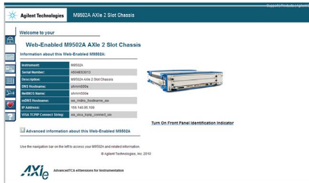
Figure 1. AXIe chassis web server
